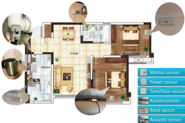
Fig. 2. In-home sensor installation places
