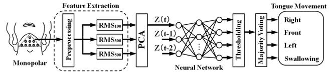
Figure 2. Tongue movement estimation algorithm.
