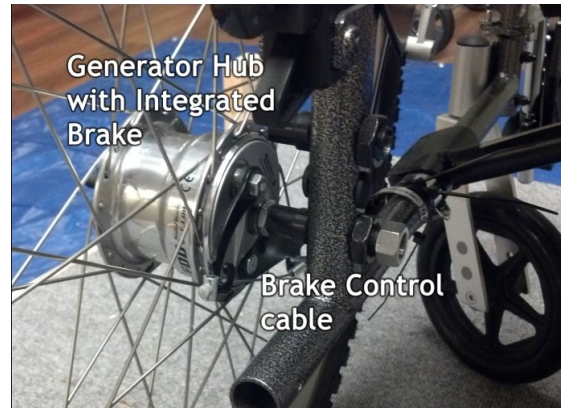
Figure 2: Hub with drum brakes and integral generator.
