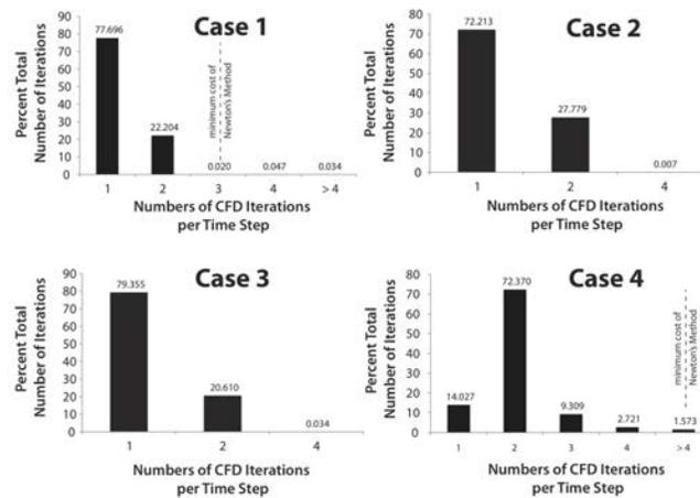
Fig. 4. Number of CFD iterations per timestep for each of the four cases. Note that in the first three cases approximately 3/4 of all timesteps required only a single CFD evaluation, while the remaining approximately 1/4 of all timesteps only required two CFD evaluations.
