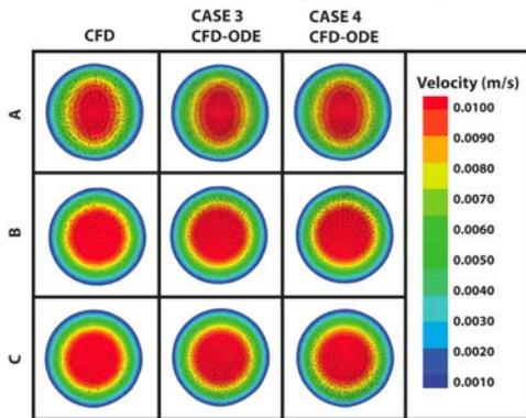
Fig. 5. Contours of velocity magnitude and vectors showing secondary flows at **peak inhalation** for the CFD and CFD-ODE Cases 3 & 4
