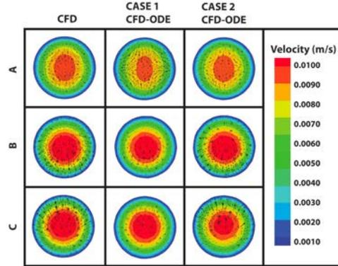
Fig. 3. Contours of velocity magnitude and vectors showing secondary flows at **peak inhalation** for the CFD and CFD-ODE Cases 1 & 2 (see Figures 1 and 2). The results are remarkably similar between each coupled and uncoupled case and the 3D CFD result.
