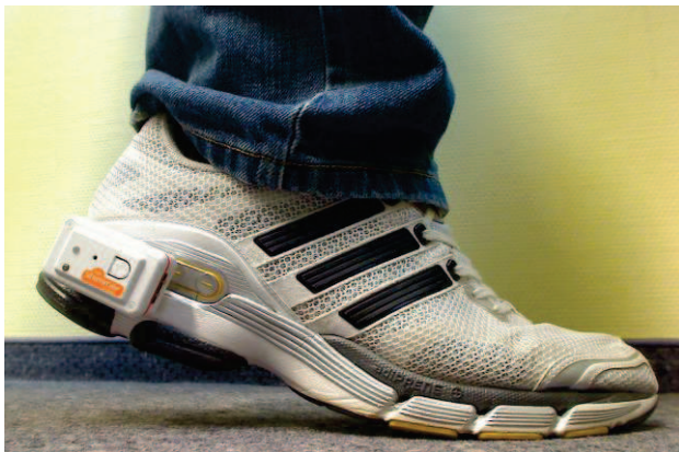
Fig. 1. Sensor setup for data capturing: sports shoe with attached SHIMMER sensor unit
