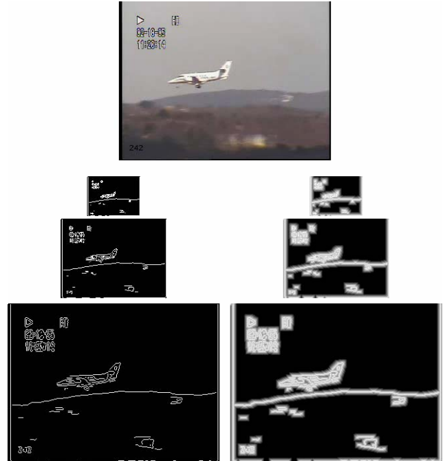
Figure 5. Images from up to down and left to right: (a) original image, (b) edge Gaussian pyramids, and (c) fuzzified edge Gaussian pyramids.
