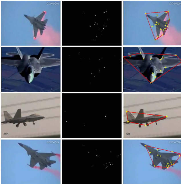
Figure 7. Images from left to right: (a) video frame t + dt , (b) the output results of classifier, and (c) the localization of target by fitting convex hull algorithm.
