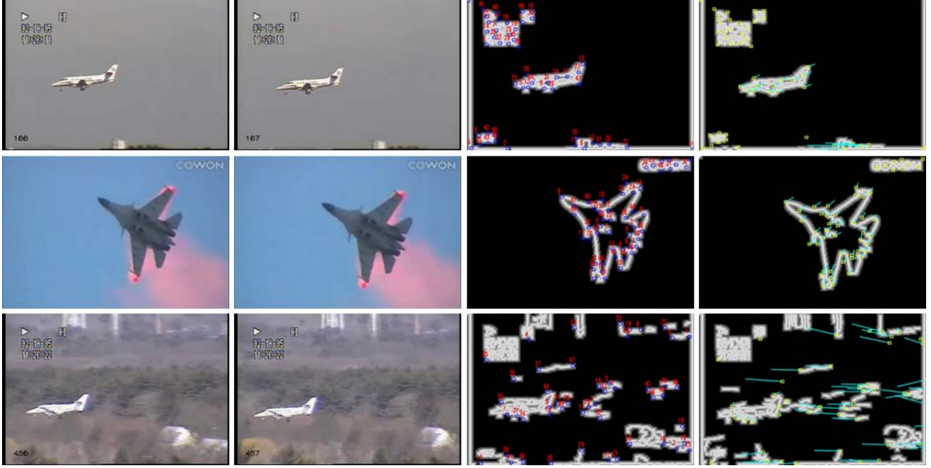
Figure 6. Images from left to right: (a) video frame t , (b) video frame t + dt , (c) the results of feature extraction from fuzzified edges, and (d) estimating flow vectors.
