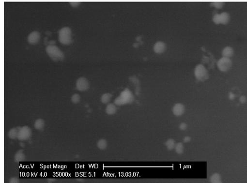
Fig. 5 – Nanoparticles after release from PEO matrix. Morphology is maintained however the nanoparticles have grown in average size.
