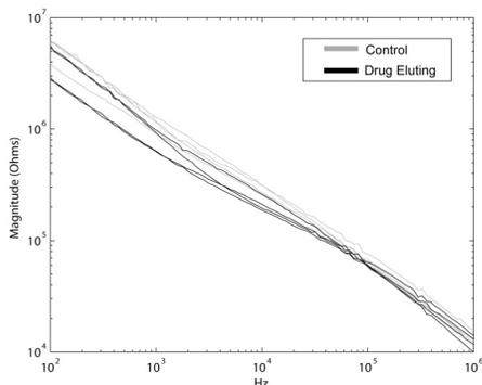
Fig. 8 - Impedance magnitude taken after 34 days (different animal subject than Figure 7). The impedance for drug eluting sites is on average lower than the control sites.
