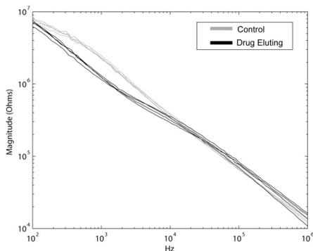
Fig. 7 - Impedance magnitude taken after 7 days. The impedance for drug eluting sites is lower than the control sites.
