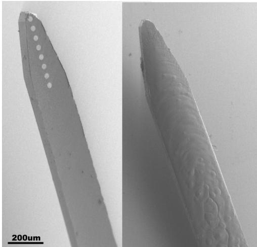
Fig. 3 - SEM image of a probe before coating (left) and after coating (right)
