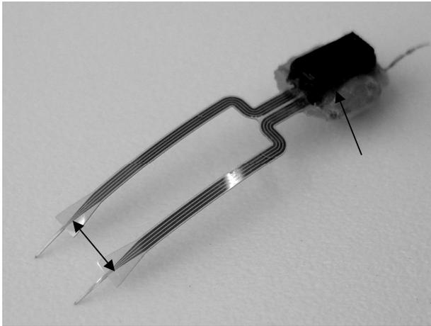
Fig. 2 The bilaterally implantable neural probe. The arrow points to the electrical connector which remains outside the animal after implantation. The double arrows span 5mm and point to the two separate probes that are implanted in each hemisphere.
