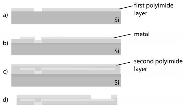
Fig. 1 – (not to scale) The neural probe microfabrication process. a) A 1.5 $\mu$ m polyimide layer is deposited on a silicon wafer and etched. b) The metal layer is deposited and photolithographically defined. c) A final thick polyimide layer (60 $\mu$ m) is deposited. c) The polyimide is etched using an oxide etch mask and d) released from the wafer.
