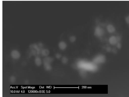
Fig. 4 – Loaded Nanoparticles suspended in saline. Average diameter is 120nm.
