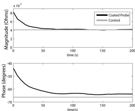
Fig 6 – An in vitro model of the impedance change after insertion in an agar model. As the PEO coating rehydrates the impedance returns to normal after only a few minutes.
