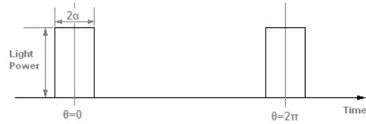
Fig. 3. Square wave signal with varying duty cycle emitted by LED.
