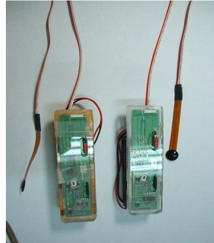
Fig. 2 The Accelerometers and Footswitches System.
