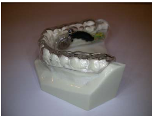
Figure 3: Saliwell GenNarino, where the stimulation electronics are embedded inside a mouth-guard like device and can be taken in and out at the patient's will.
