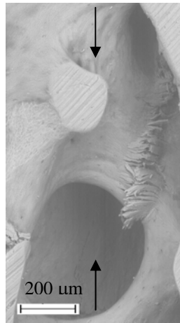
Figure 8: Failure of a single trabecula, \sigma/E_0 = 0.0067 , cycle 1,747.
