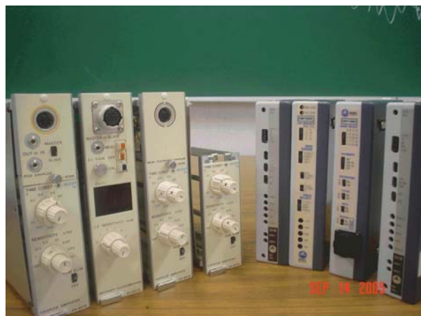
Figure 2: NIHON KOHDEN and BIOPAC Systems Inc. amplifiers for measuring physiological signals. From left to right: (a) PCG, (b) Cardiac Output, (c) Peripheral Pulse wave and, (d) Respiratory curve.
