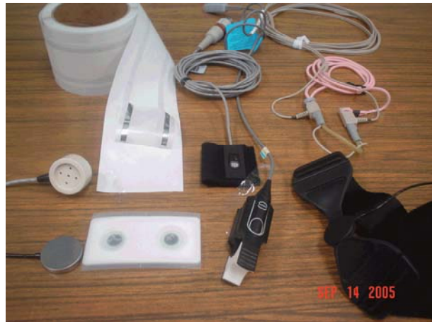
Figure 1: NIHON KOHDEN (top) and BIOPAC Systems Inc. (bottom) transducers for measuring physiological signals. From left to right: (a) PCG, (b) Cardiac Output, (c) Peripheral Pulse wave and, (d) Respiratory curve.
