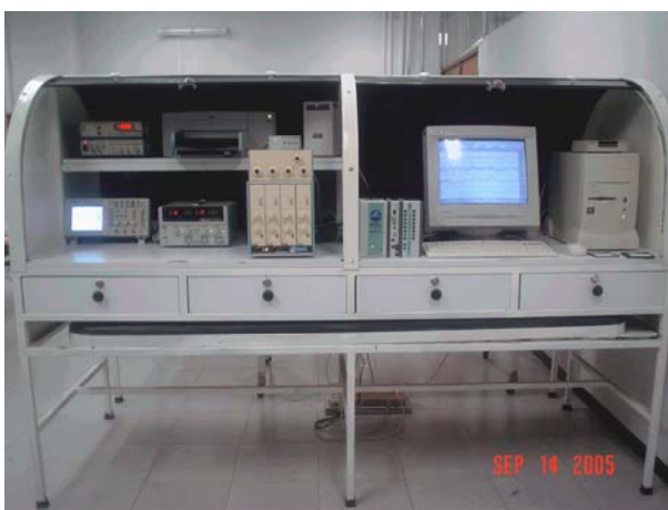
Figure 4: A workstation outfitted with equipment from Tables 1 and 2. From left to right: (a) electronic measurement, (b) printer, (c) basic system composed by a NK polygraph, four NK bioelectric amplifiers, and a MP150 system from BS, (d) computer with data acquisition and processing software.
