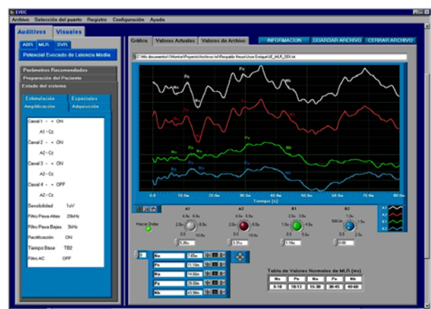
Figure 6: A Virtual Instrument that a student programmed to remotely control the Neuropack Sigma, a clinical system for measure Auditory, Somatosensorial and Visual Evoked Responses. Reader can see the Medium Latency Auditory responses obtained by the VI.
