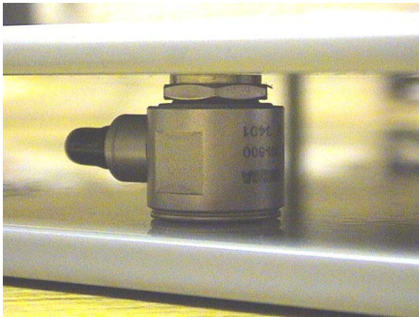
Figure 5: Main sensor of the QSCG measuring equipment - detail of the solid-state accelerometer between measuring metal plates.
