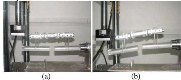
Figure 4: Cantilever bending test of unilateral fixator with serrated joints: (a) Before, (b) After lateral bending load
