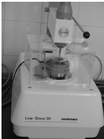
Figure 1: Couette type flow chamber of the rheometer Low Shear 30 Contraves between the coaxial cylinders – pair of electrodes
