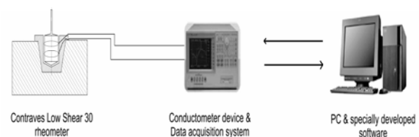
Figure 3: Principal electrical scheme of the device for acquisition and processing of data (Data acquisition system) from the rotational viscometer Contraves Low Shear 30
