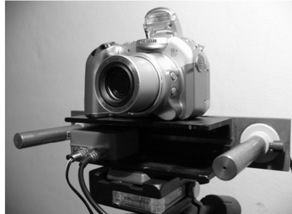
Figure 3: Tripod attached with device for setting cameras on the same optical axis.
