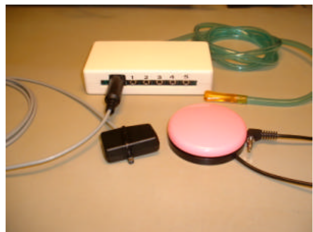
Figure 4: The complete system with a built-in sip-and-puff unit, five contacts for push-buttons, the motion sensor and one push-button in front.
