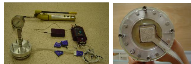
Figure 4: Calibration equipment for capacitive pressure sensors (left); a pressure sensor pad when subjected to hydraulic pressure during loading (right)
