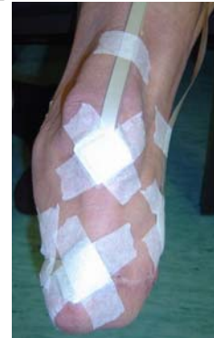
Figure 1: Test locations for contact pressure measurements [6]
