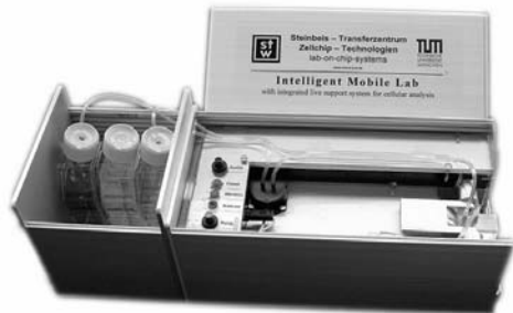
Figure 2: Intelligent Mobile Lab device. The front part (size: 210mm x 105mm x 90mm) includes all the electronics, sensor chip, pump system and controls. The back part (size: 90mm x 105mm x 105mm) includes only the reservoir tanks.
