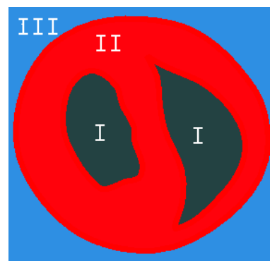
Figure 4: Domain decomposition. No adaptivity during element generation was allowed in area II.
