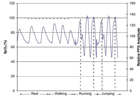
Figure 5: Effect of motion artifacts on PPG waveform and SpO 2 recordings from the forehead using an elastic headband attachment.
