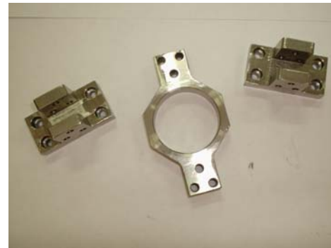
Figure 2: Photo of Load Cell and the Supports.
