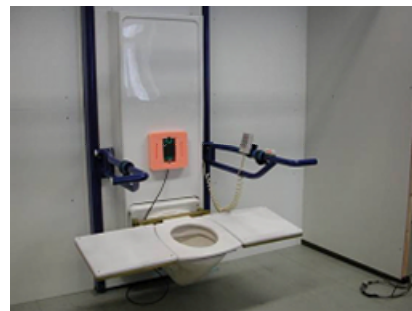
Figure 4: Prototype with extended seat, grab bars and ultra sonic distance sensor behind the user's back.
