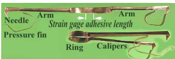
Figure 7: Thin-plate ring-caliper type extensometer.
