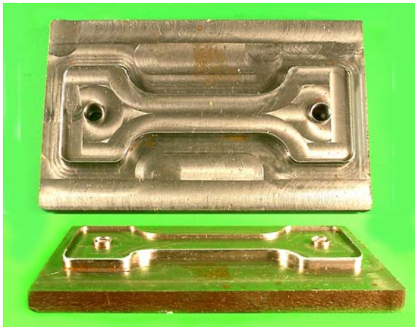
(a) Cutting die used for polyurethane sheet blanking
