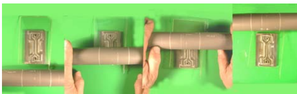
(b) Roll-cutting procedure
