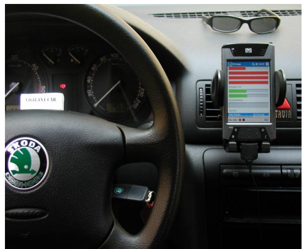
Figure 3: New experimental equipment, real-time visualisation of estimated indicators.
