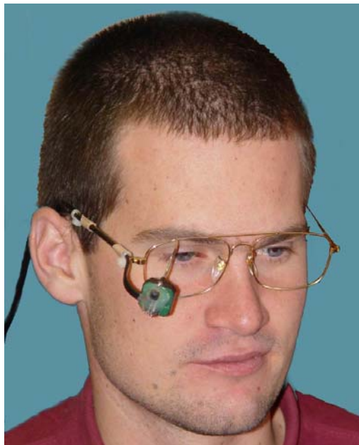
Figure 5: Location of the camera in the system I4Control ®
