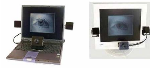
Figure3: System for monitoring reflected light by a photodetector
