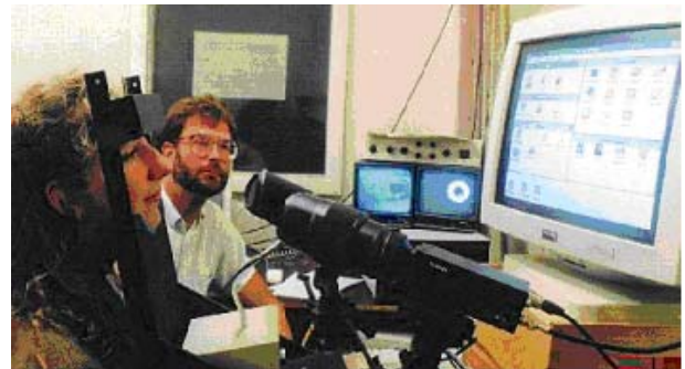
Figure 4: System for videoculography
