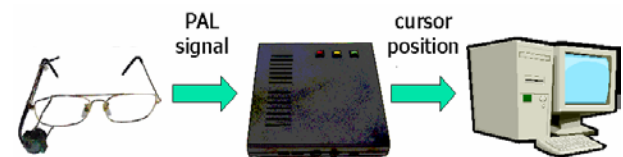
Figure 6: Basic block structure
