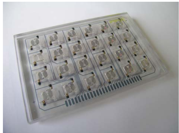
Figure 7: Mounting with sensorchips and electrically contacting of the 24-well-microplate
