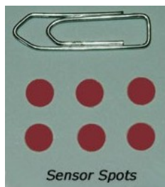
Figure 2: Optically read-out sensorspots for oxygen [5]
