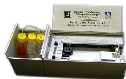
Figure 8: Intelligent Mobile Lab (IMOLA) for the monitoring of living cells
