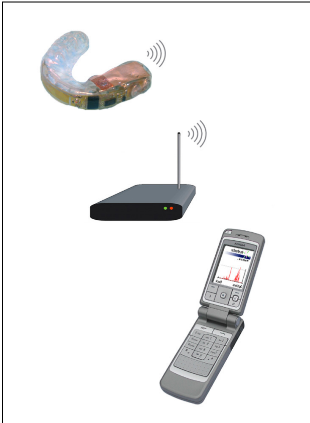
Figure 3: The telemetric bruxism diagnosis System
