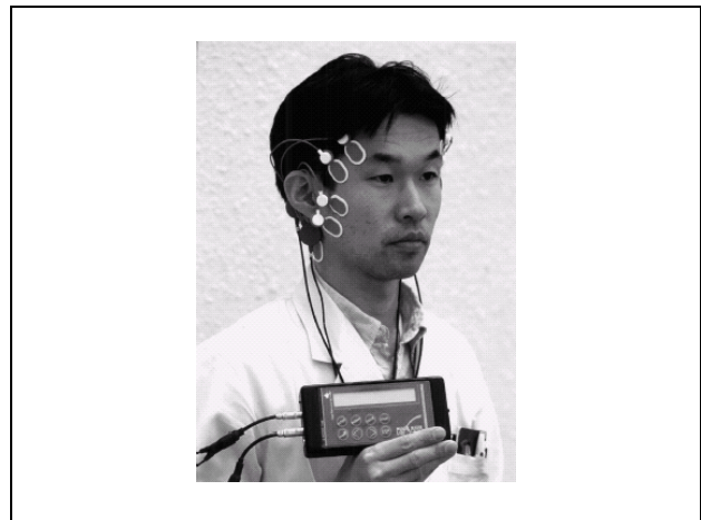
Figure 1: Measurement with EMG Electrodes in daily life [6]
