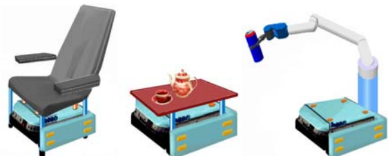
Figure 1: Typical combinations of MOVEMENT-modules for moving people and objects
