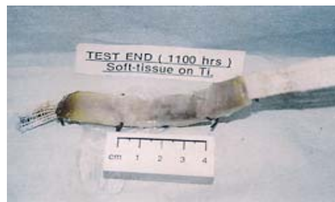
Figure 7: Soft tissue against titanium
