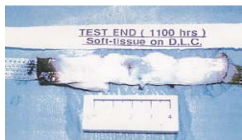
Figure 9: Soft tissue against DLC coated titanium
