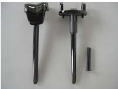
Figure 11: Components of knee replacement DLC coated for Royal National Orthopaedic Hospital Metal implants in contact with blood such as stents, are thrombogenic. DLC coatings can reduce blood coagulation. On transcutaneous prostheses, in which the
