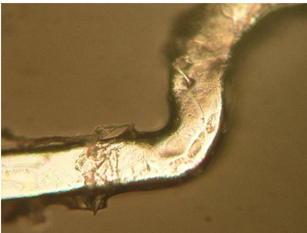
Figure 5: A strut with the peeled off coating
