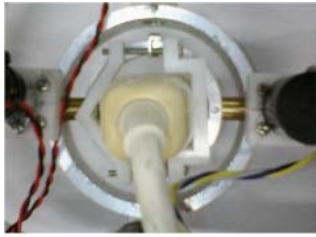
Figure 3: Inner ring with the pentagonal-shape vice
