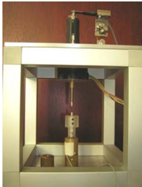
Figure 2: Micro-compression device, showing the displacement sensor on top, the stepper motor and its interface suspended from the platform and the container for the scaffold with the piston and load cell at the bottom. The coupling between the piston and the stepper motor axis stands next to the container.
