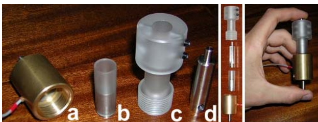
Figure 3: Container holding the scaffold and its assembly that is inserted into the \mu CT scanner. Left: a Base containing the load cell b Watertight sample holder c Body with radiolucent window and grub screws for fixation of piston d Piston. Middle and right: Complete assembly.
