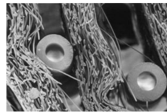
Figure 2: Close up of the non-woven polyester matrix and the oxygen capillaries with void spaces for plasma flow in between.
