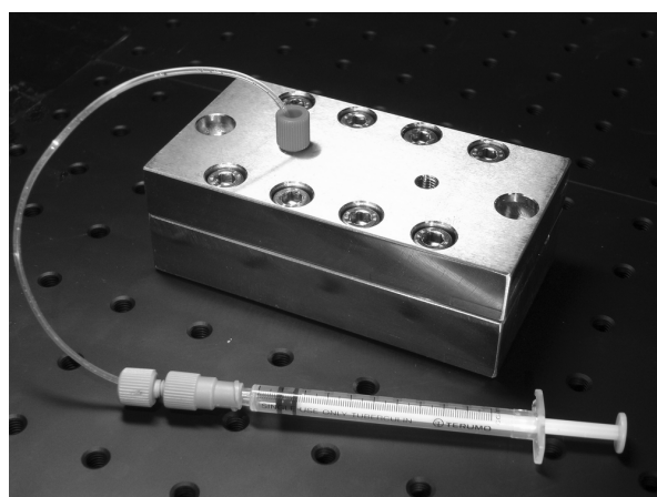
Figure 2: Photo picture of the device. The PMMA microtrench chip and the glass microarray slide are sealed together by steel clamps. 1 ml syringe is used to pump the target sample.
