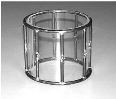
Figure 2: The built lowpass birdcage coil
