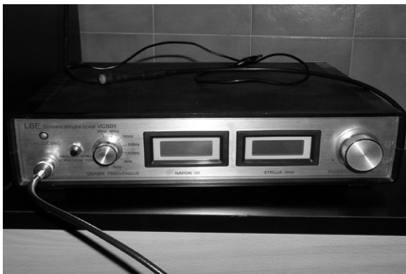
Figure 1: Sinusoidal constant current source VCS01 designed for the experiment. On the central position of the front panel are LCDs for RMS voltage and current intensity.
