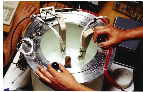
Figure 3: Experimental 2D setup for USCT. The white tank is filled with water and contains the object to be imaged. Two unfocused ultrasound transducer arrays are manually moved on a ring with 12 cm diameter to simulate 100 sending and 1600 receiving positions in one circular layer around the object.
