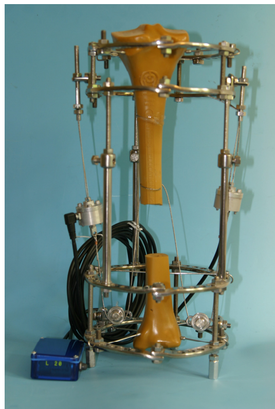
Figure 5: External fixator for bone segment transport equipped with the monitoring system and two force sensors
