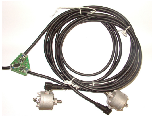
Figure 6: Cable assembly with embedded signal processing for two force sensors
