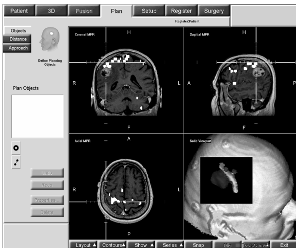
Figure 1: Export of fMRI activations (white dots) to an SNN navigation system. The information was used to segment the precentral gyrus.
