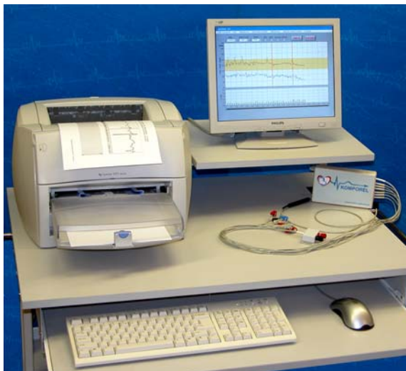
Figure 1. System for recording and analysis of bioelectric signals from maternal abdominal wall.
