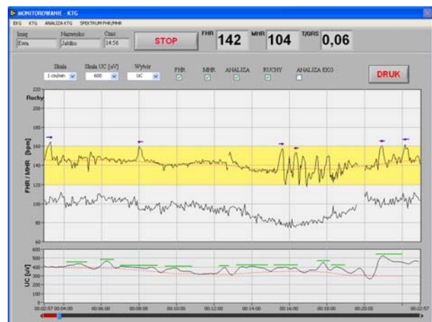
Figure 6. System window with traces and graphically presented results of their analysis: detected FHR accelerations patterns, contractions recognized in UC signal.
