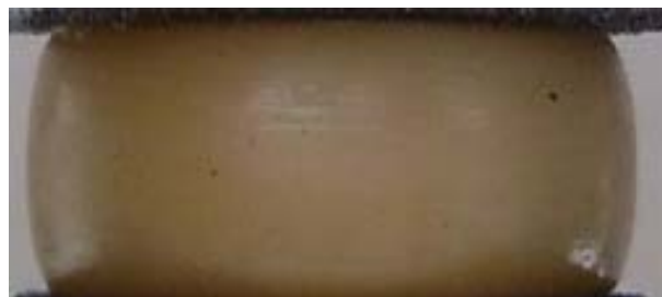
Figure 6: Photo taken from the side view of pure GelFlex specimen after compression
