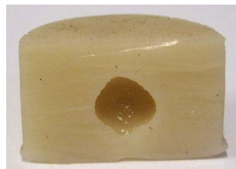
Figure 2: The slice of elastomer used in this experiment, showing gas trapped inside the GelFlex phantom
