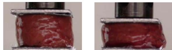
Figure 10: Compression test (before and after) on liver
