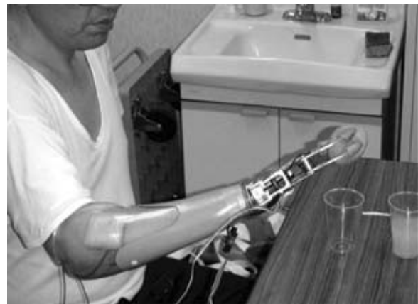
Figure 5 Photograph of the handling of a soft object with the prosthesis.
