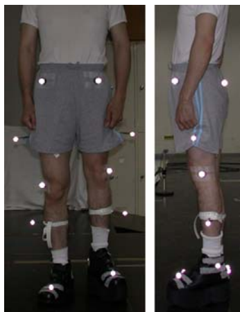
Figure 1: The subject is wearing the footwear and 15 light-reflecting markers are set according to the Helen-Hays method [5].
