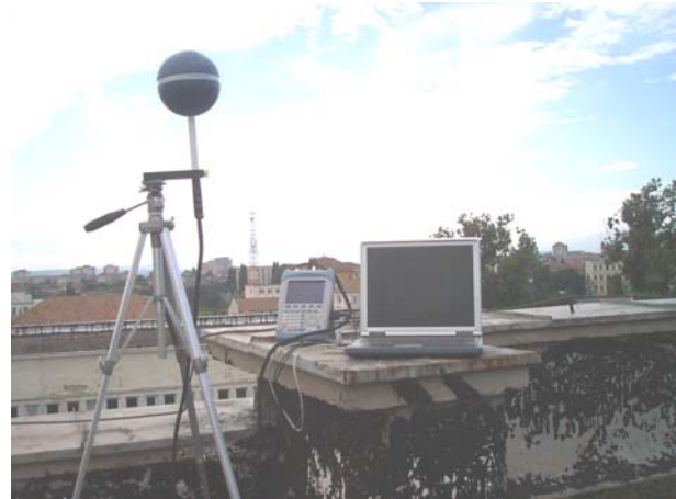
Figure 1: The R&S TS-EMF system used for measurements
