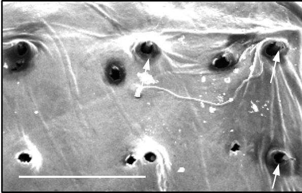
Figure 9: Scanning electron micrographs illustrating the ability of wet-etch microneedles with frustum-shaped tips to penetrate the epidermis; arrows highlight microneedle tips seen protruding through the human epidermal membrane Scale Bar = 1mm
