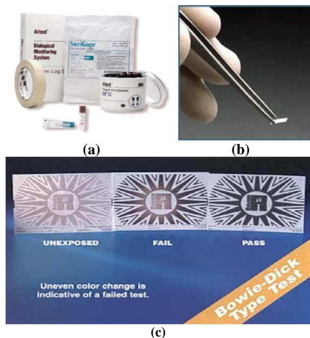
Figure 5: Several commonly employed sterilisation indicators: a) Attest Biologic Indicator, b) Mini spore-strips and c) Bowie-Dick type test Indicators.
