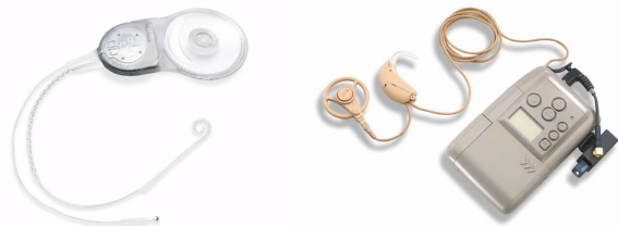
Figure 1: Nucleus implant CI24R and Sprint™ bodyworn processor.
