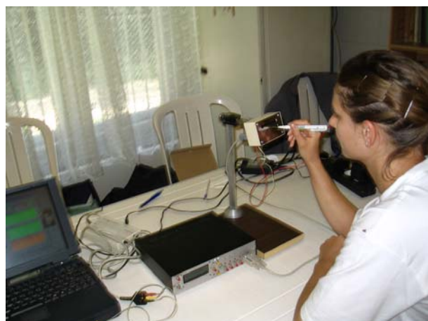
Figure 1. Special device for hand tremor assessment and reaction time measurement.
